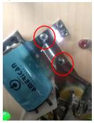
4) Install the left E.O.S. with the Brown/Blue wire as shown using 2 screws and a nut bracket. Reinstall the 2 Phillip screws securing the E.O.S. Bracket once E.O.S. is attached.
