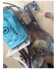
5) Route the Brown/Blue wire to the lower left switch board (3<sup>rd</sup> slot from the right) and solder the black ground wire to an adjacent switch ground. Use wire ties to dress wires.
