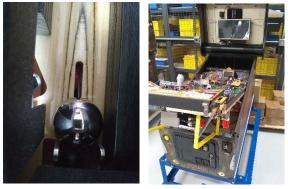
Remove the three 11/32 nuts, remove and disconnect the planchette and loosen the three Philips heads
