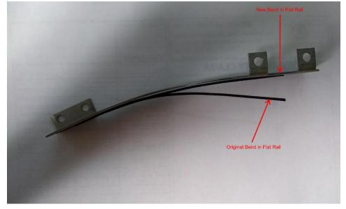
Remove the 7/16" rubber and insert the 3/16" rubber. The post closest to the flat rail will no longer have a rubber on it. The goal is to have the flat rail touching the post without the rubber on it.
