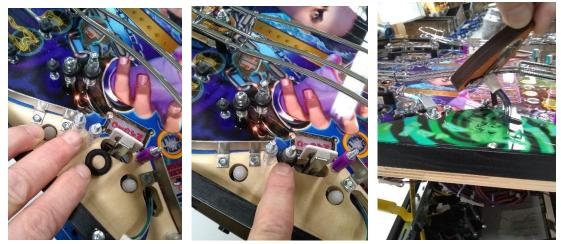
Reinstall the gate, plastic and planchette. Test to ensure the ability to hit all three stand up targets from the shooter lane.
