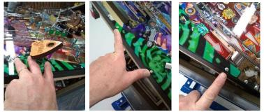
Remove the two ¼" nuts holding the gate on and remove the gate.
