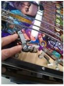
Remove the two Philips and two ¼" screws
