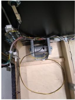
Using the 4 like screws fasten the shaker motor to the pinball. See picture.
