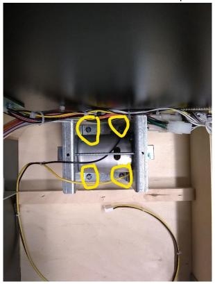
Install shaker motor cover with the remaining screws <u>be mindful that the cable is not in the path of the spinning weight.</u> Then remove wire keeper and route shaker motor cable under it and replace screw. *See picture.*
