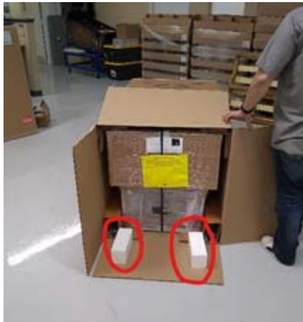
Figure 2.2 Carton View After Laying On Side
