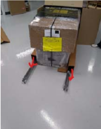
Figure 2.5 Remove Bottom Corner Protectors
