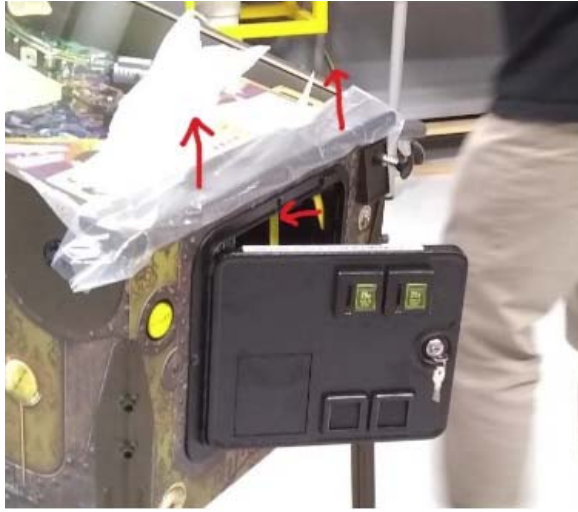
Figure 2.16 Securing Head in Place
