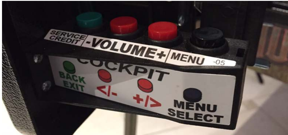
Figure 3.2 Service Menu Navigation Buttons
