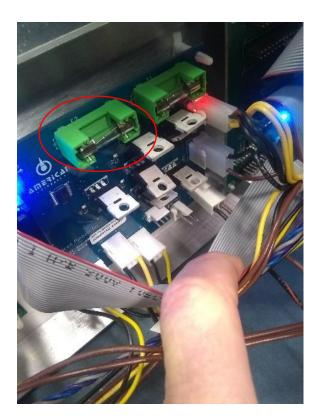
8) Dress new wire with wire ties. Re-install PCB cover with 2 thumb screws from step 5.
