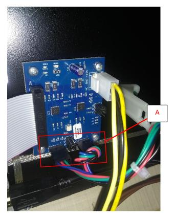
2) With the power off switch the two stepper motor inputs.
