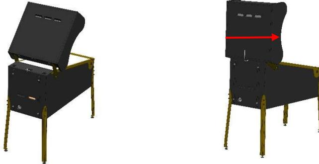
Remove the keys from the ball shooter. One set is for the back box, the other set is for the front coin door. Open the coin door and move the lock down handle to the left and pull up on the front trim. Remove the trim from the clear protector. Pull the glass off and follow the instructions under the glass.
