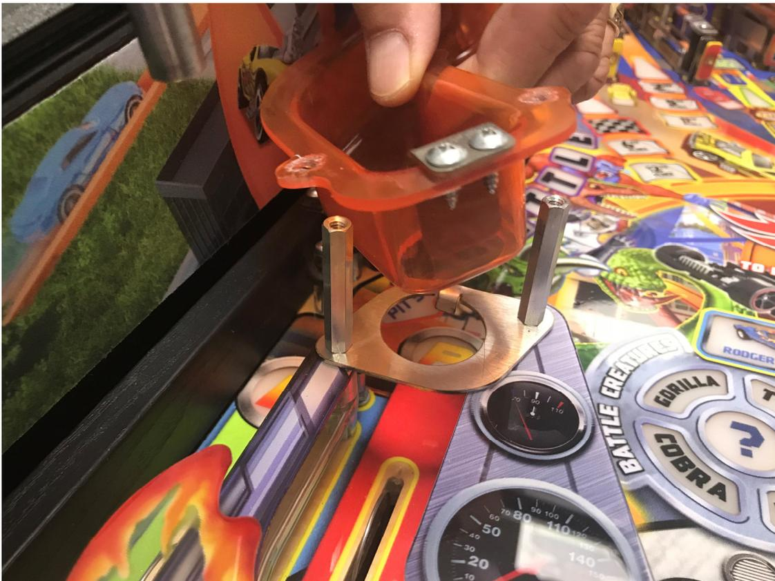
**Step 6.)** Place a washer over the slot in the orange ramp and then fasten the screw back into the hex post, using your #2 Phillips screwdriver. Repeat this step for the other slot in the orange ramp exit. Make sure the fasteners are secure, but do not overtighten.
