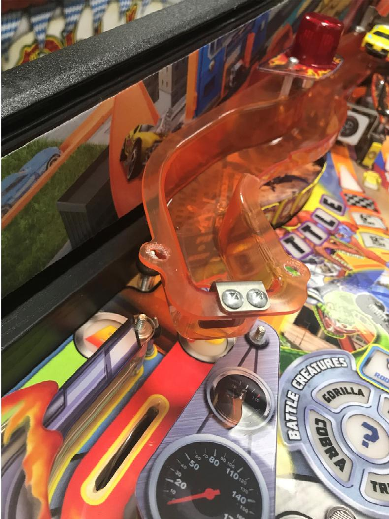
**Step 3.)** Gently lift the orange ramp, and place the left Ramp Exit Plate as pictured below, with the tab in the center hole pointed downward.
