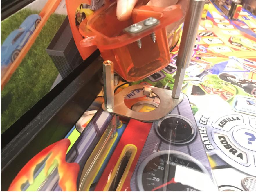
**Step 5.)** Carefully align the Ramp so the slots in each side of the ramp line up with the holes in the hex spacers.
