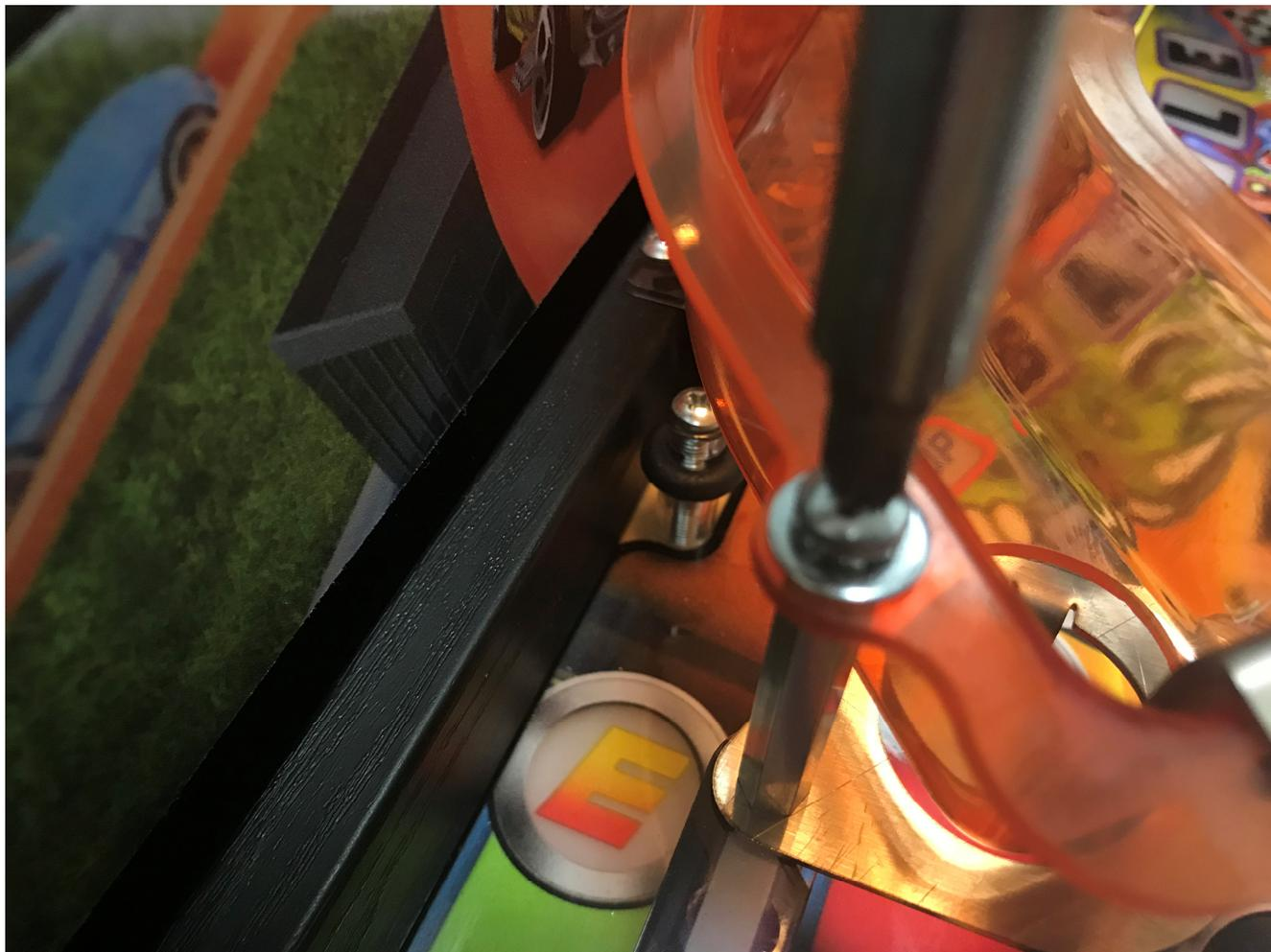
This is how the Ramp Exit Plate should look when installed from the top-down view.
