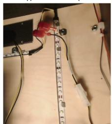
**Note:** for 2021 built Houdini games, there is already a mate-n-loc connector at the end of the LED strip to plug in the topper cable.
