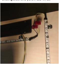
**Step 7**. Plug the mate-n-loc Y connector to the topper cable and T-tap ends
