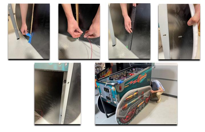
With both sides of the tank attached to the machine, plug the open ends of the LED connector cables [B] into the controller [D]. Plug one end of the adapter [G] into the controller and the other into the wall. The LEDs around the tank treads should turn on.
