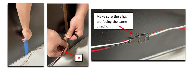
Pull the wires up the channel, cover with the plastic cable cover [C], and line it up with the predrilled holes in the tank. Screw in the cover with woodscrews [F] and a phillips head screwdriver.
